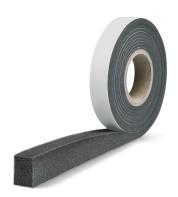
possibility of humidity and mould formation. The WINS Fix external self-expanding tape is a self-adhesive open-cell polyurethane foam-based tape for sealing between the window and the internal, plastered surface of the jamb. It is flexible and compensates for the movement of the structure. Compatible with substrates made of aluminum, PVC, wood, silicates, concrete, cellular concrete, ceramic hollow bricks, brick, plaster, etc. Does not react with PU foam and MS Polymer based sealants.
